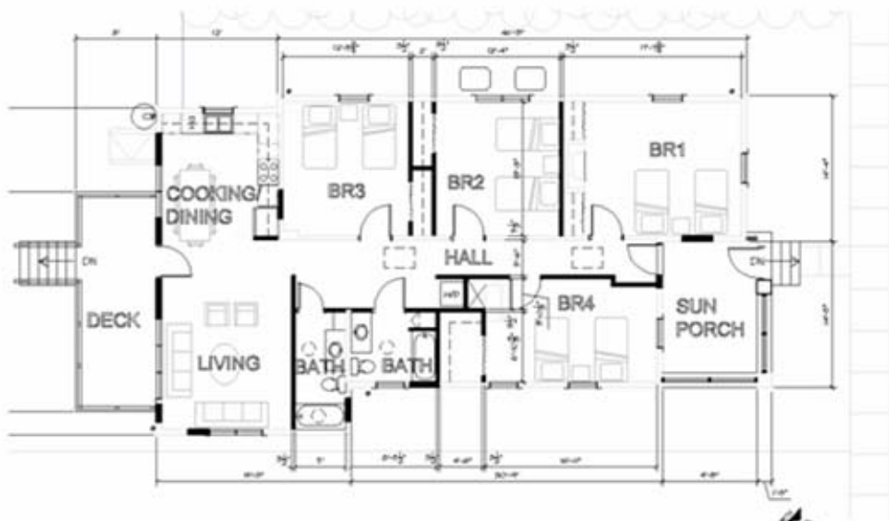
RENOVATION FIRST FLOOR PLAN SCALE: 1/8" = 1'-0"
